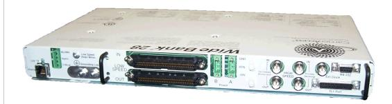
The Wide Bank<sup>®</sup> 28 provides a high-density, lowcost DS3-to-DS1 or DS3-to-E1 service delivery solution that offers hitless protection and hitless maintenance as well as dual redundant DS3 options. It featured a carrier-quality NEBS Level-3-compliant design, and is OSMINE-compliant w/TL1 provisioning and management.
