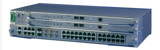
TraverseEdge™ 100 contains a Fully integrated SONET/SDH ADM and Ethernet switching in a 2RU shelf. TE 100 offers an affordable delivery of Ethernet Fast Ethernet, Gigabit Ethernet, DS1/E1 and DS3/ E3 services from a compact system. The multiplexers' Full Ethernet over SONET/SDH feature set includes GFP, HO/LO VCAT and LCAS.
